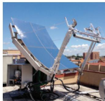
*Fig.1 Asymmetrical parabolic trough*
