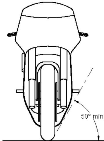
B.2.1.3 The minimum distance between the prototype in upright position and the road surface must be of at least 100mm in rest situation. This measurement will be done with the prototype unloaded (without the rider), but with all the equipment and liquids for its operation.
