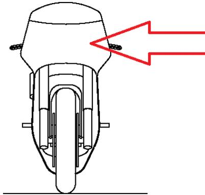
B.11.1.2 In the front number, the minimum dimension of each character must be 140mm in height and the minimum stroke width of each character must be 25mm. The minimum distance between characters must be 10mm.
