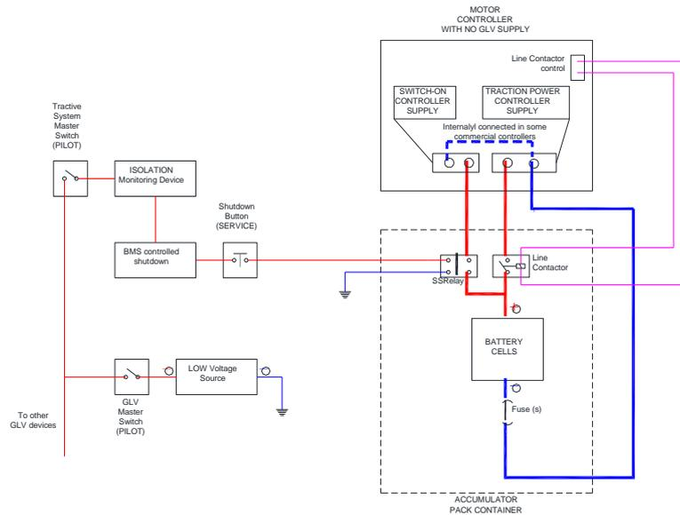
**Diagram 2: Contactor directly controlled by the controller**
