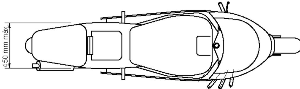
B.2.1.8 The maximum width of the fairing shall be 600mm.
