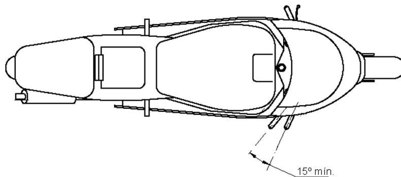
B.8.1.2 The turning angle must be limited with stoppers on both sides. These stoppers should be made of nylon, aluminum or materials of similar hardness. Neither the chassis, or any other part of the prototype may act as a steering stopper.
