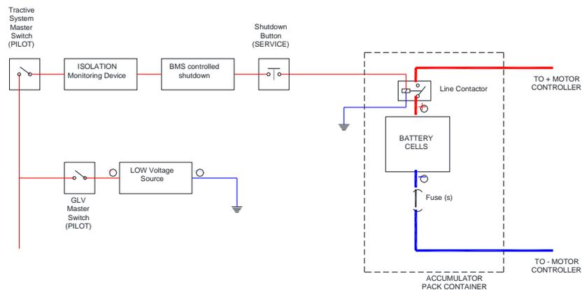
**Diagram 1: Contactor directly controlled by the disconnection circuit**
