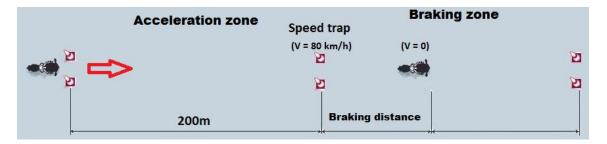
Graphic description of Test 1: Brake Test
