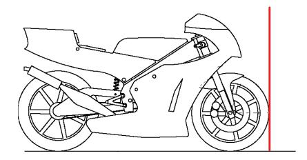
B.2.1.5 Rear limit: No element of the prototype shall protrude from the vertical line drawn tangentially with respect to the external circumference of the rear tire.
