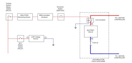
Diagram 1: Contactor directly controlled by the disconnection circuit
