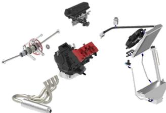
The engine map and the exhaust system had been realized with the purpose of having a better response from the engine at low and medium RPM and to be specifically adapted to Formula SAE requests.
