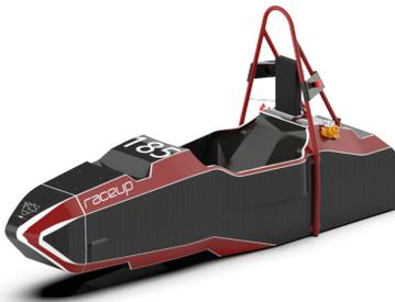
The carbon fibre monocoque, that we develop, maximizes stiffness and safety. With a weight of just 23kg it also allows us to be extremely high-performing .
