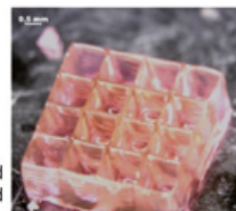
Fig. 4. 3D printed gelatin scaffold
