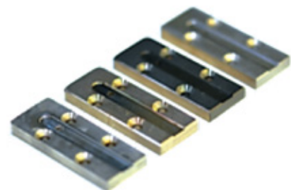
Figure 2. Different mold inserts with different coatings. From the left to the right: uncoated mold insert, ALD coating, DLC coating and SiO x coating.
