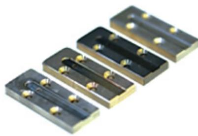
Figure 2. Different mold inserts with different coatings. From the left to the right: uncoated mold insert, ALD coating, DLC coating and SiO<sub>x</sub> coating.
