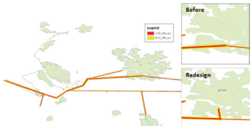
Figure 2 Pipeline network near Manchester city: CO 2 consequences due to full bore rupture and redesign network to improve the safety near center of city.
