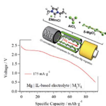
Figure 3 - Concept and performance of a magnesium secondary battery employing an ionic liquid-based electrolyte and the highly active δ-MgCl<sub>2</sub> salt
