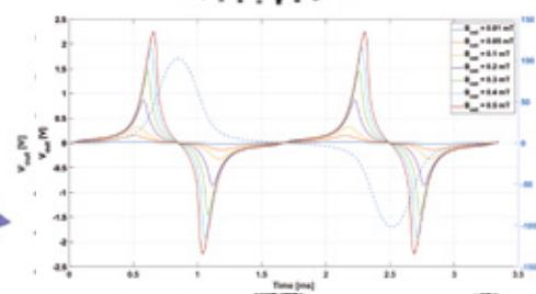
Figure3: simulated excitation current and raw output signal
