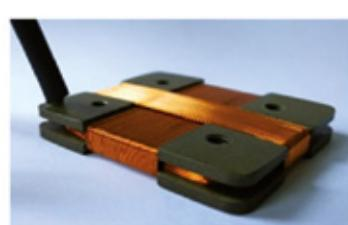
Figure1: new three-axes pick-up sensor (left) and system layout (right) of the RFXmod2 experiment
