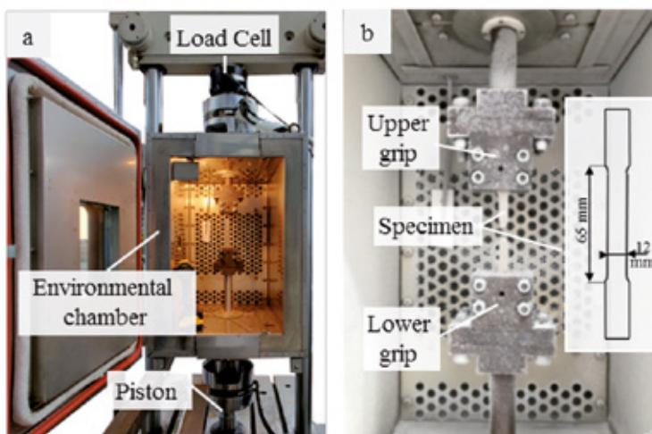
Fig.1: Experimental equipment for sub-zero temperature tests.
