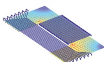
Figure2: FEM analysis of a miniaturized fluxgate sensor
