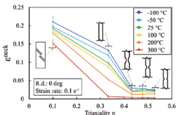
Fig.2: Necking locus at varying temperature.
