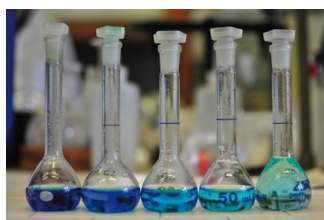
Figure 2. Methylene blue discoloration after PAC treatment.
