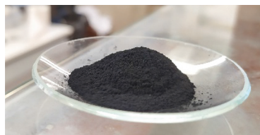
Figure 1. Powdered activated carbon obtained from spent coffee grounds.
