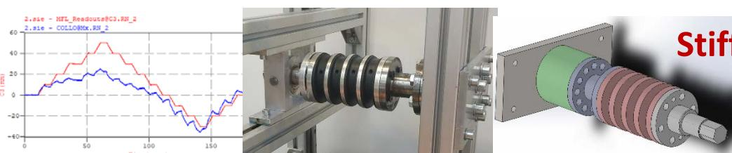
**Stiffness properties of the biofidelic Hybrid III neck: bench and pilot tests development**
