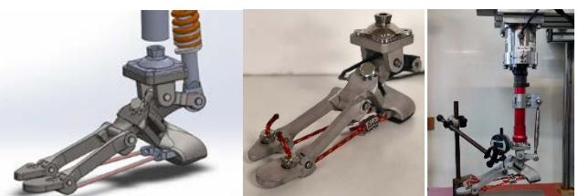
**Construction and Validation of a Biofidelic foot/ankle/leg prosthesis for gait simulation on footwear**
